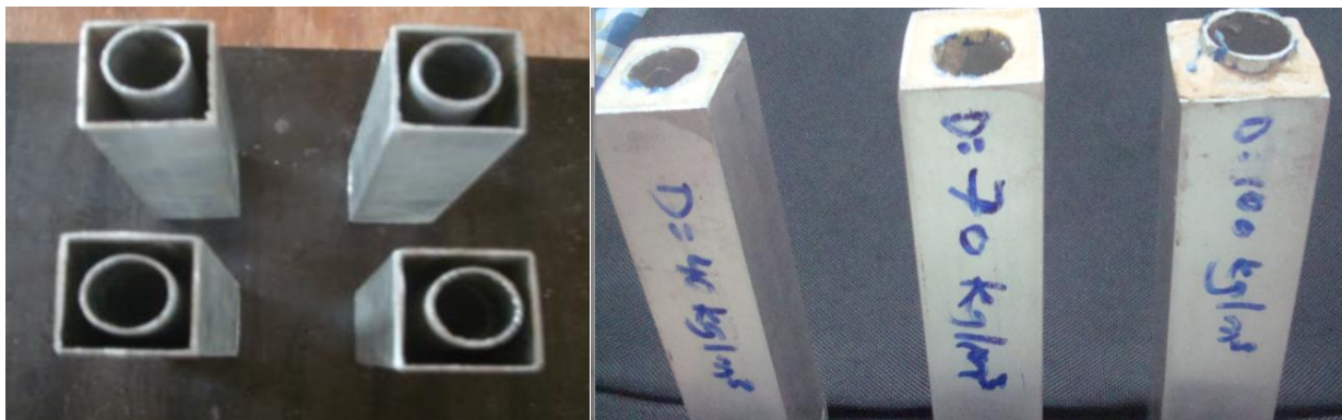
Fig 3.1.1 Experimental specimen of Empty and filled Concentric tubes
