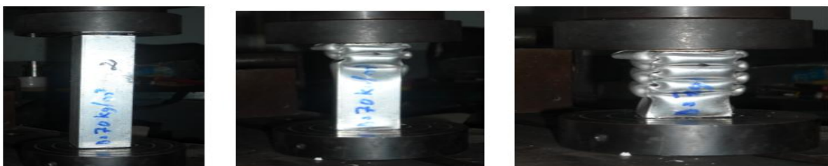
Fig 3.2.1.1 Deformation modes of foam filled (70kg/m 3 ) Concentric tube
