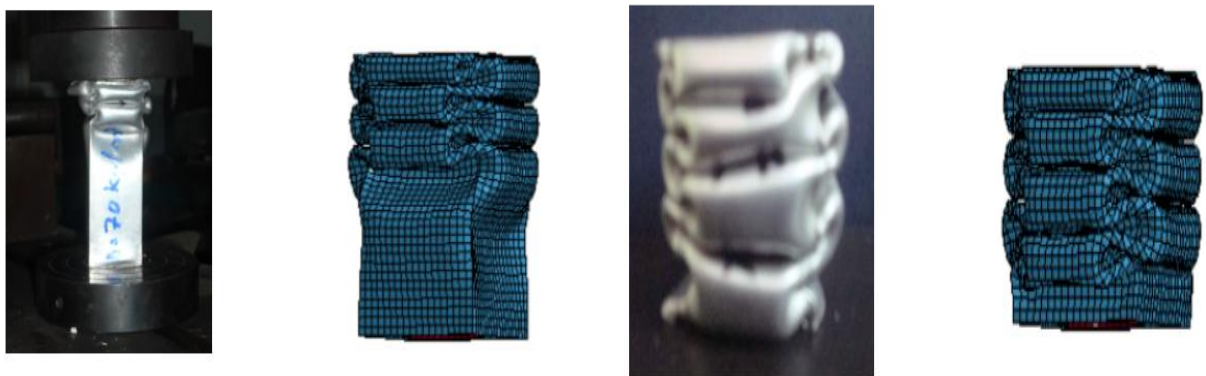
Fig 4.1 Deformation modes of Experimental and numerical simulation respectively
